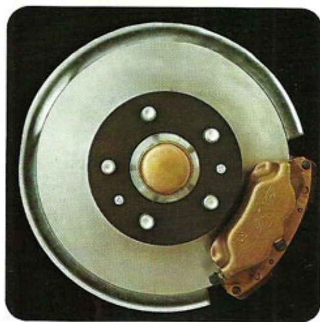
Four-wheel disc brakes are standard. The front discs are ventilated on the 242GT and 260 Series.
