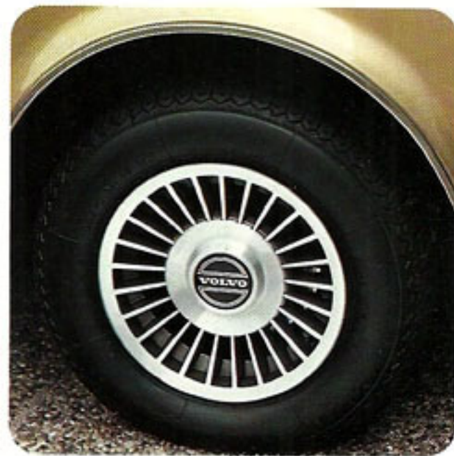
Volvo's 25-spoke light-alloy wheel is included on the 264GL and 262C. It's also available on the 240 Series.
